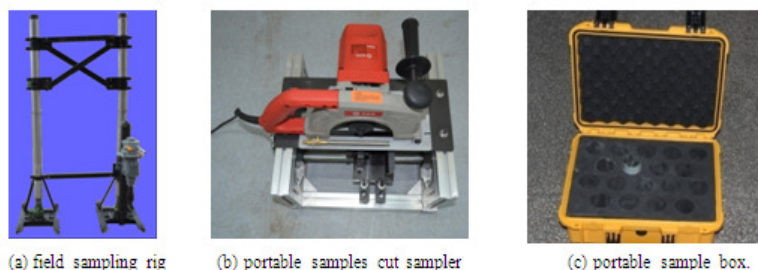
Fig.3 Undisturbed samples sampling system.
